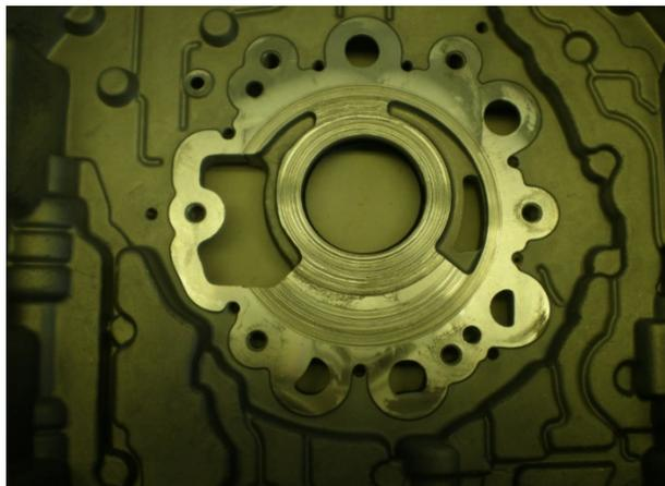
Fig. 4. Seats of leakage failure
